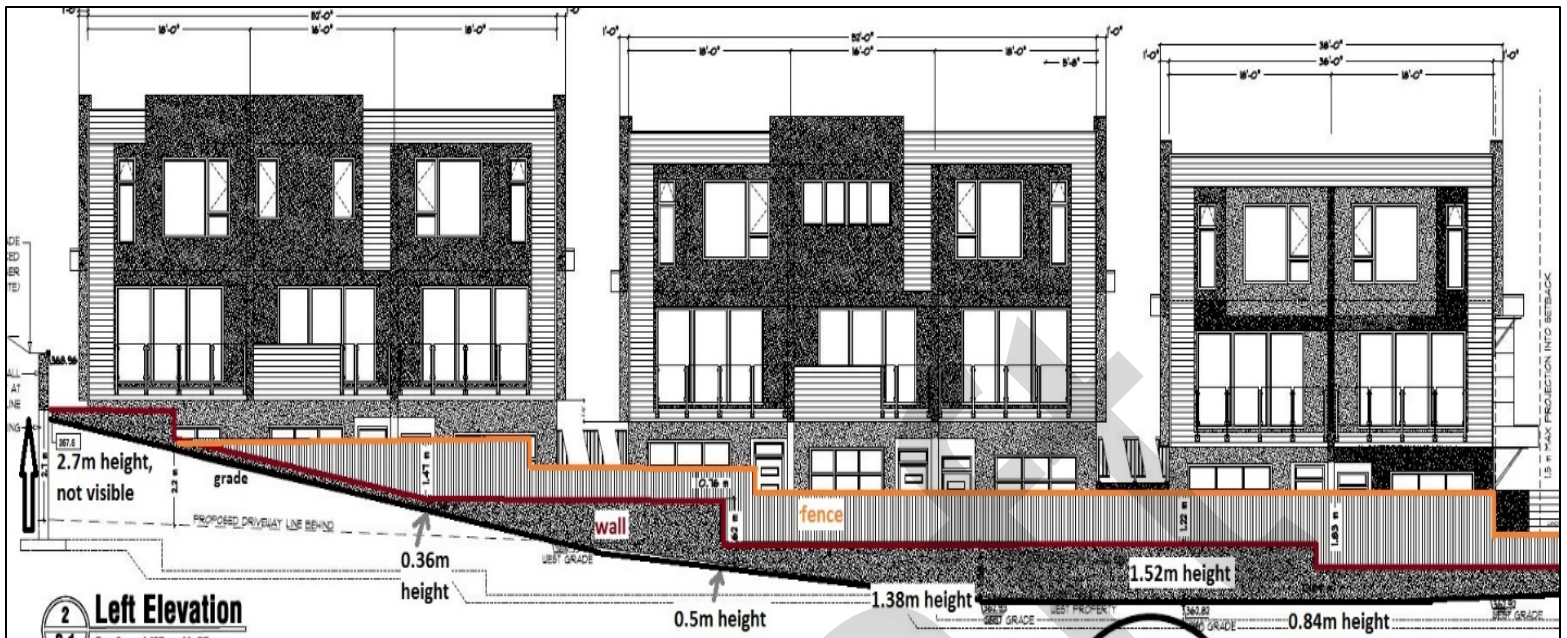
Figure 12: Retaining Wall along west property line
